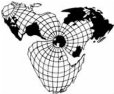
图 5 以南极为中心的哈默等面积分瓣投影 (Spilhaus 和 Snyder, 1991) Fig. 5 Hammers equivalent interrupted projection in the center at South Pole
