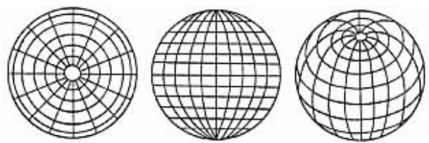
图1 正轴、横轴、斜轴方位投影 Fig. 1 Diagrammatic sketch of azimuthal projection of normal, transverse and oblique
