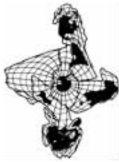
图 7 一种分割的以南极为中心的横轴正弦曲线等面积分瓣投影 (Spilhaus, 1990) Fig. 7 Equivalent interrupted projection of transverse sine curve in the center at South Pole
