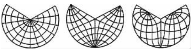
图2 正轴、横轴和斜轴圆锥投影 Fig. 2 Diagrammatic sketch of conic projection of normal, transverse and oblique
