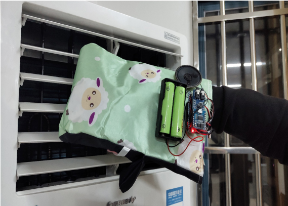
图10 自适应模糊PID电动车手套控温保暖系统实物 Fig.10 Electric vehicle gloves of temperature control and warming system based on adaptive fuzzy PID
