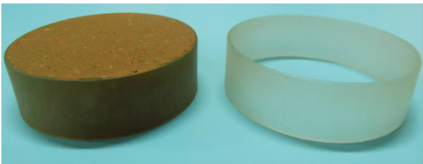
图 4 聚砜塑料制成的环刀样及环刀 Fig. 4 Cutting ring samples and cutting rings made of PSU
